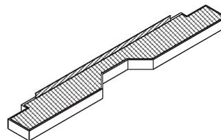
**Bumpers - Outrigger Ball Hitch Recessed Treadplate**
