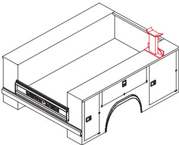
**BMS1HD-ADJ - Heavy Duty Adjustable Crane Boom Support**
