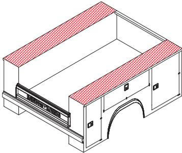
LCW - Liner, Treadplate Compartment Wall \*
