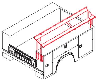
LRF - Ladder Rack (Side Mounted, Flat Type)
